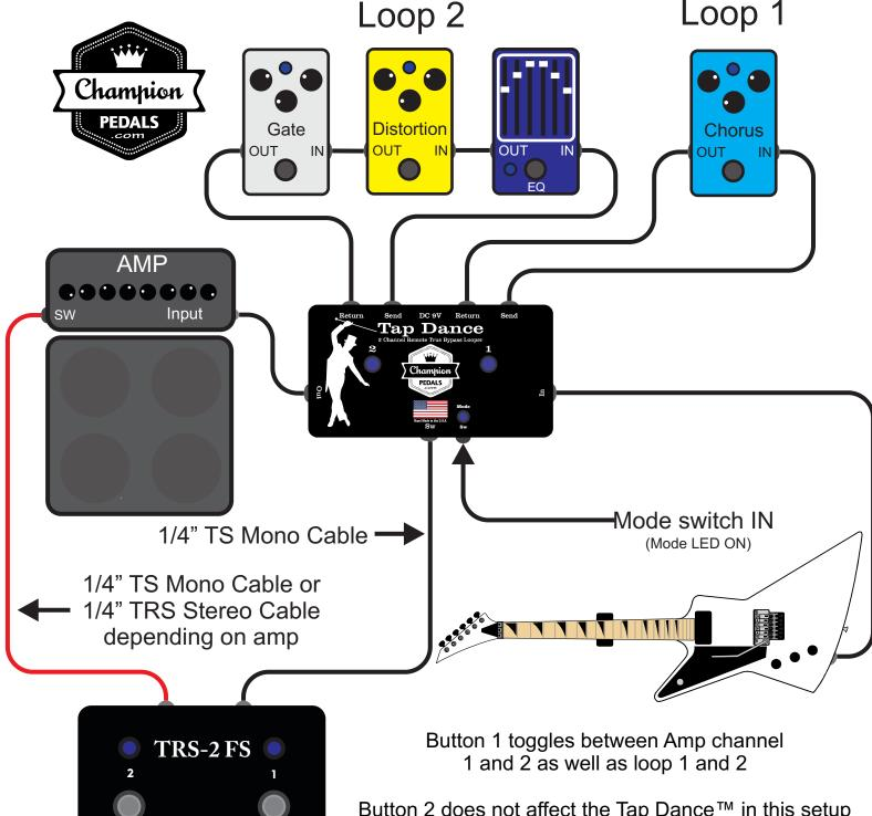
The switching jacks in the TRS-2FS are completely isolated so there will be no ground issues
